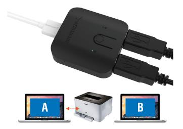
**6** - The LED light will indicate which computer currently has control of the attached peripheral
